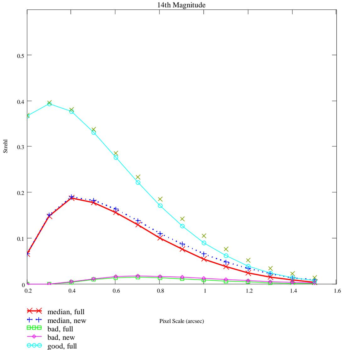
**Figure 4.9 - Delivered Strehl as a Function of WFS Pixel Scale**
